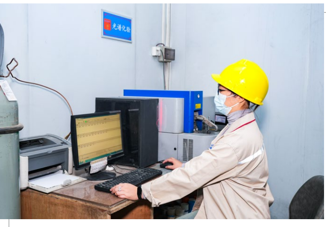
采用德国斯派克台式光谱前材质化验 Using German Spike desktop spectroscopy for material analysis
