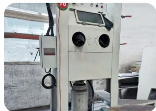
喷砂Sand blasting
